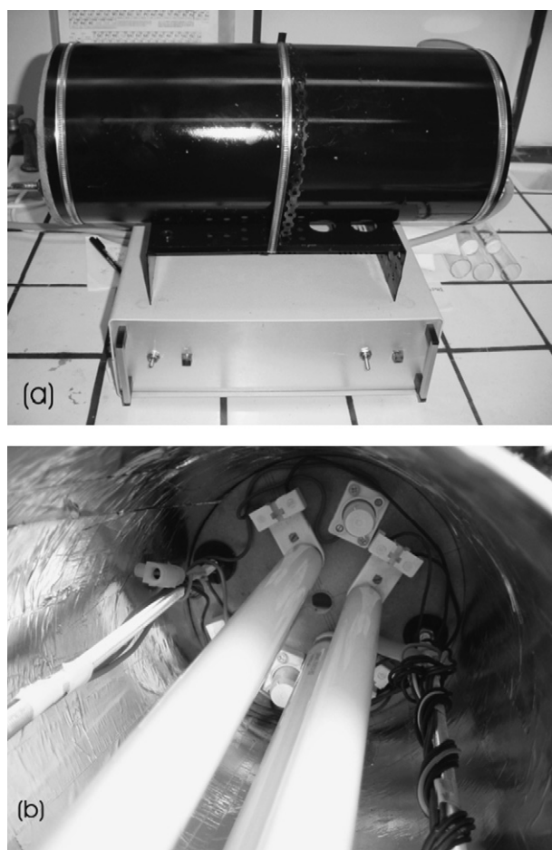
Fig. 1. The photocatalytic packed bed reactor (PPBR) used in this study: outer (a) and inner (b) views.
